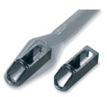
It is essential to lock the line securely for the compensator to work properly. Forsheda mooring compensators are equipped with locking elements at both ends which are vulcanized into the compensator. The lock elements, which are injection-moulded and made of polyamide 6 (nylon). lock the line securely without causing wear.
