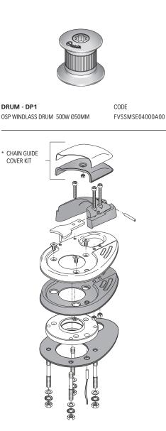
COMPLETE BASE - DP1 OSP WINDLASS BASE SERIES DP1 COMP \* OSP CHAIN GUIDE COVER KIT DP1 CODE FVSSBDP110C00A00 FVSSCPSCDP10A00
