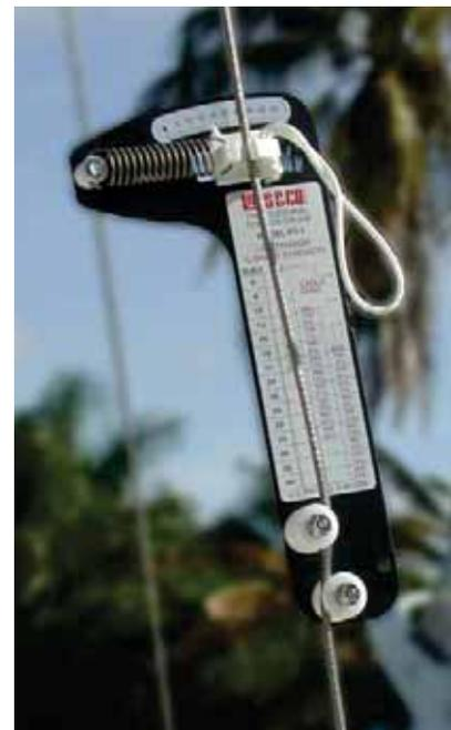
Each model covers a tension range of approximately 5% to 25% of the breaking strength of the wire and is designed and tested to provide an accuracy of plus or minus 3% at mid-range.
