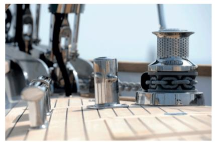
All of our calibrated chain is supplied with a certificate of conformity and test. This confirms that the chain has been subjected to a proof load and our in-house batch testing ensures that the chain can withstand the minimum breaking load.
