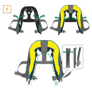
Unpack lifejacket by opening burst points and running your finger around the jacket. Run the zip to the left side (operating head side) ready for re-packing.
