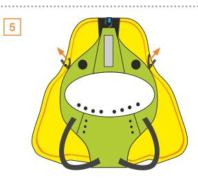
Fasten velcro through punched holes in bladder fabric.
