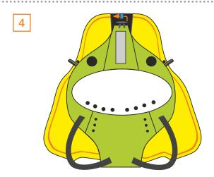
Place hood on top of jacket and pass toggle through loop.
