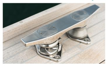
JOY is designed and realized in Stainless Steel AISI 316 L with particular attenction in over dimensional protocoll and attention to the sea side condition, it can be use for vessel from 50 to 70 feet. It is well utilized and installed in bow as in stern singularly or in couple.
