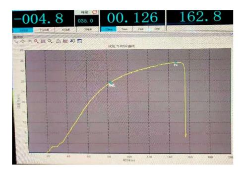
According to the testing results, product 01.740.08 has the maximum breaking load capacity35KN, screw of the product breaks, casting curve surface deforms.
