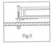
When mounting on bulkhead, hatch or cabin roof, always use distance sleeve and mounting sheet so that there is an open space between the hub and the nearest surface.
