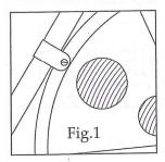
When mounting direct against the tube of the pulpit, change the screw of the drum to a 50 mm screw. The drum can of course pass the pulpit and be adjusted with a mounting sheet.
