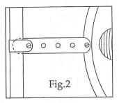
If you cannot reach the pulpit, use a mounting panel and a clip, which should be connected by a 16 mm screw, a nut and bolt.
