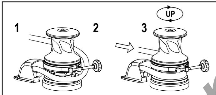
1. Insert the chain into the hole and fix to a safe point.
