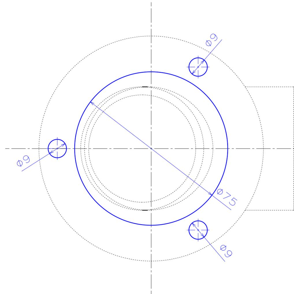
Overall Chain Pipe Contour over deck
