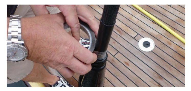
PSP Marine Tapes have produced a tape to protect expensive race sails from wear by reducing friction on contact points of the rig. Unlike anti chafe, rig wrap is supplied self wound (without a liner) and will stretch to coil wrap around standing rigging, terminals, forestay, backstay, spinnaker poles, spreaders and any other areas of contact, preventing wear to sails and friction to sheets and guys etc. The tape will stretch and coil wrap around all areas on board.
